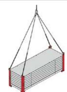
Stacking device ease the crane handling and ensures easier site stacking. Moreover, the stacks can be easily moved with a fork- lift. The stacking device enables quick and safe sticking of 8 panels of a particular size.
